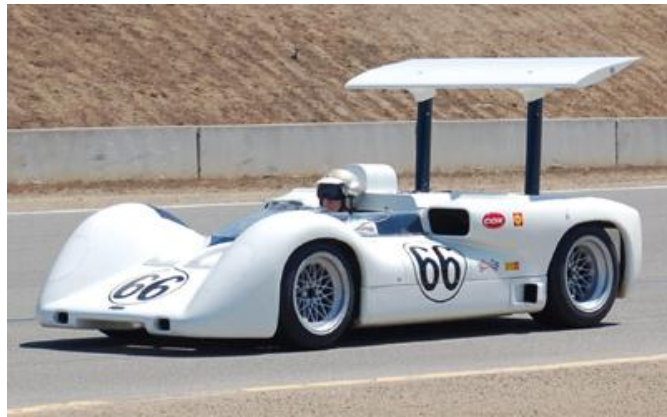
Figure 1: Jim Hall's Chaparral 2E, the first elevated wing mounted on struts [2]
